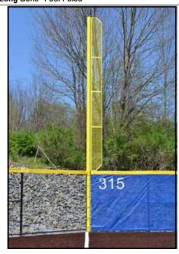
Long Gone® Foul Poles are manufactured from 4" or 6.625" outside diameter aluminum pipe and are available in standard above ground heights of 15', 20', 30' and 40'. All foul poles are powder coated yellow, utilize ground sleeves with corresponding caps or a base plate mounting system for a semi-permanent installation, and are available with or without a wing.
