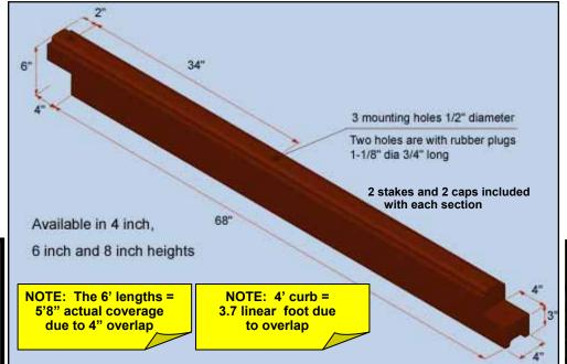
Please note: The 4" wide sections are grooved and can be stacked to create desired height,. However, the 3" W is not stackable. 3" W lengths of curbing are not grooved for stacking.
