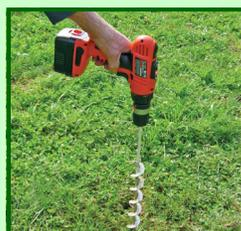
3. Mark and drill holes for poles with optional 18" auger.
